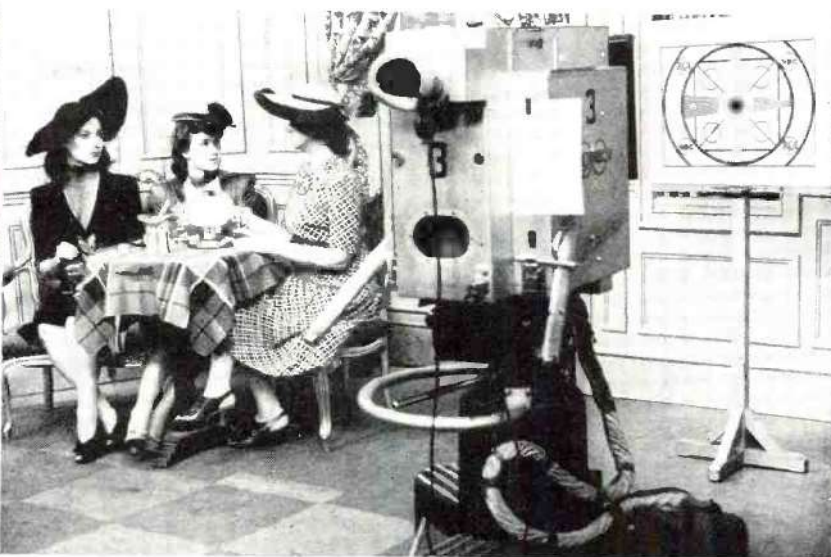
The camera is focused on the test pattern designed to serve the purpose of stand-ins. This is more accurate, serves special television needs and saves wear and tear on the cast. The various technicians: cameramen, light men, technical director, video man, etc., line up their controls and the camera for deflection with a peculiar chart. Sharpness is still not perfected.
