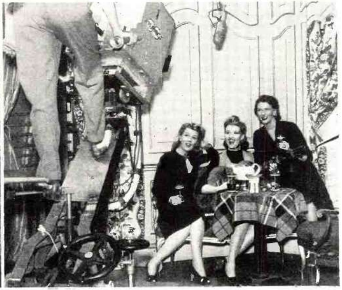
The camera shown is fixed on a hand-operated dolly that performs gymnastics which make a wide range of camera angles possible. A dolly man drives the cameraman around the studio and hoists him up and down. Other lifts are electrically operated.
