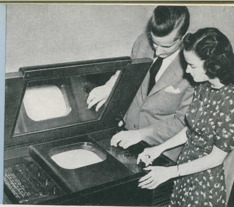
RCA television receiver with lid raised to show how the image screen is reflected in a mirror under the lid.
