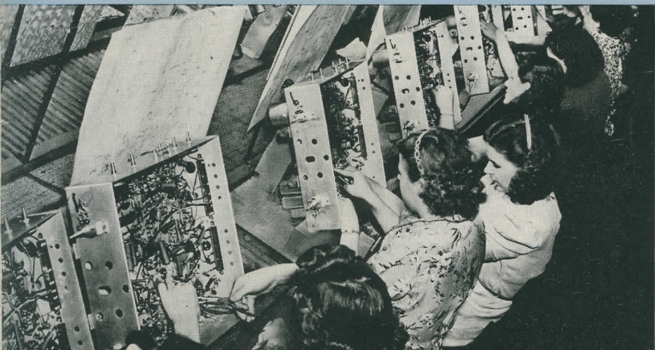
A section of the television receiver assembly line at the RCA-Victor factory at Camden showing operators wiring chassis from the underside.
