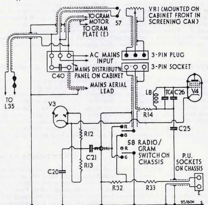
This diagram to be used in con-junction with T.18 sound diagram on Section 12 (3), additional components are:
