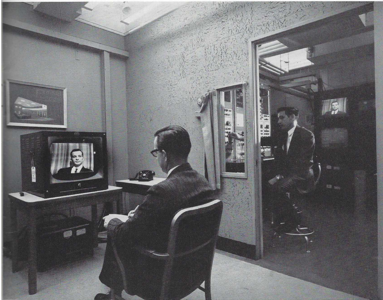
The variable-parameter television system laboratory. R. H. Rosasco, at the control panel, adjusts picture parameters which the author, A. D. Hall, in the viewing room, judges them according to standards of clarity, brightness, etc.
