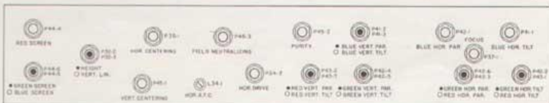
Fig. 2—Deflection chassis front controls.
