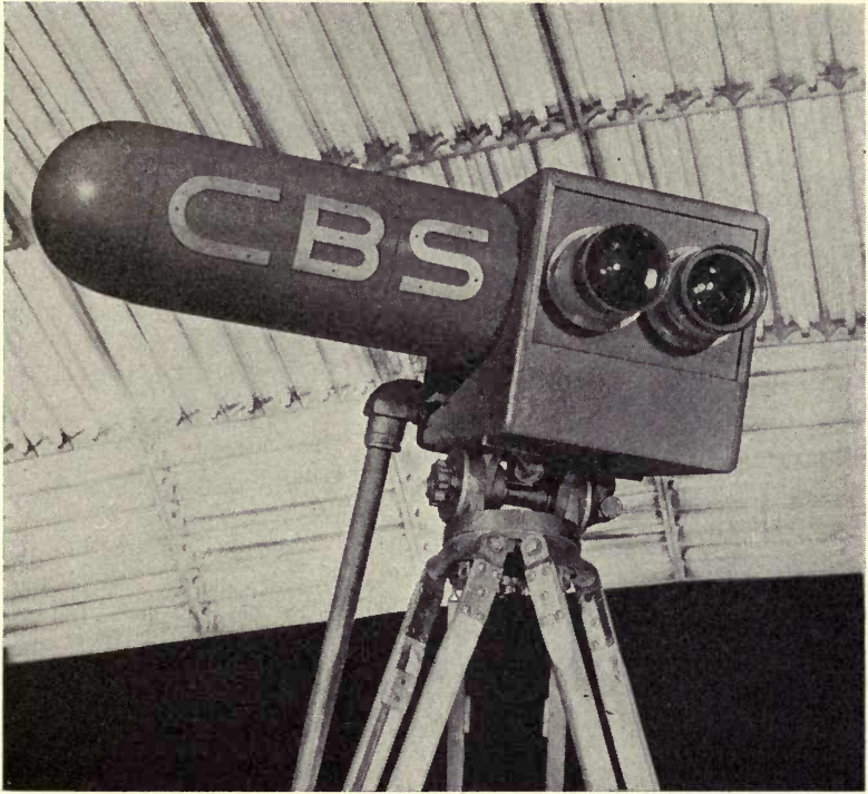
Color camera used in 1940-41 demonstrations at CBS. The revolving color disk is in projecting tube at right of camera.
