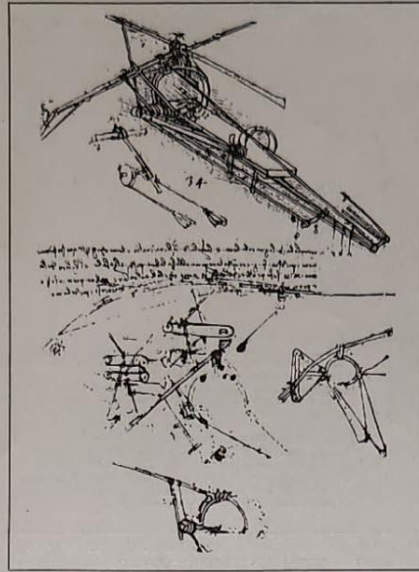
FLYING MACHINE USING ARMS AND LEGS, OPERATOR LYING PRONE, MANEUVERING TAIL BY OPERATOR'S HEAD
