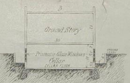
Fig. 2.—After alteration, with the cellar space made available for manufacturing purposes.
