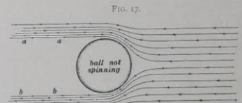
FIG. 17. Showing how a rapid stream splits when it flows past a ball.
