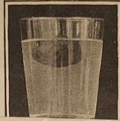
A COMMON HEAVY STONE FLOATING IN A GLASSFUL OF BROMOFORM.
