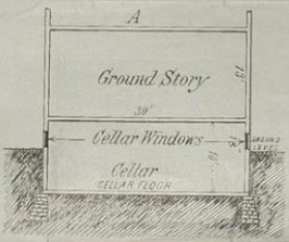
Fig. 1.—Original state of the building, with dark cellar space.
