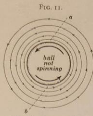
FIG. 11. Air whirl produced near a spinning ball—air everywhere at rest except in so far as it is affected by the spinning ball.
