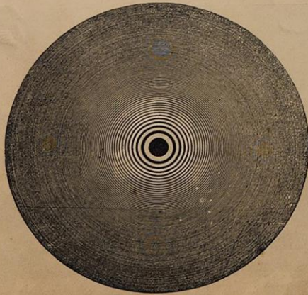
PHASE-REVERSAL ZONE-PLATE. A copy of this figure, in the form of a transparency on glass, can be used instead of a lens.
