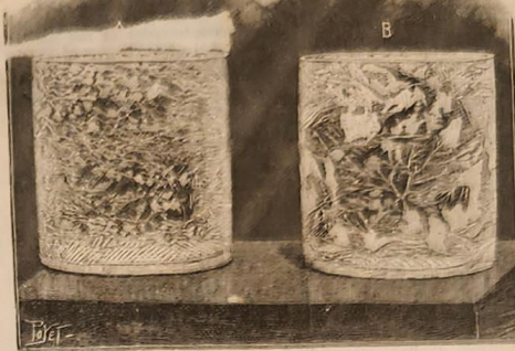
FIG. 1.—A. GLASS VESSEL ETCHED BY THE ACTION OF GLUE AND ALUM. B. GLASS VESSEL ETCHED BY PURE GLUE.
