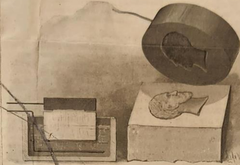
METHOD OF ELECTRO-ENGRAVING AND SAMPLE OF WORK.
