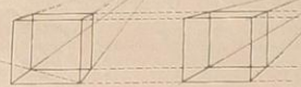
Fig. 1.—Showing method of stereoscopic drawing. The dotted lines represent the penciled construction lines.
