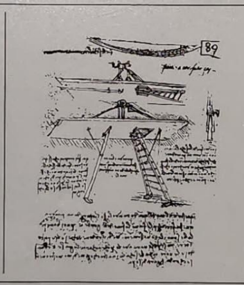
FOLDING LADDER WITH SHOCK ABSORBER FOR LANDING, SHOWING COLLAPSIBLE MECHANISM
