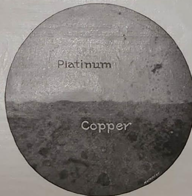
Fig. 8.—Microphotograph of a copper-platinum weld. Magnified 1,000 times.
