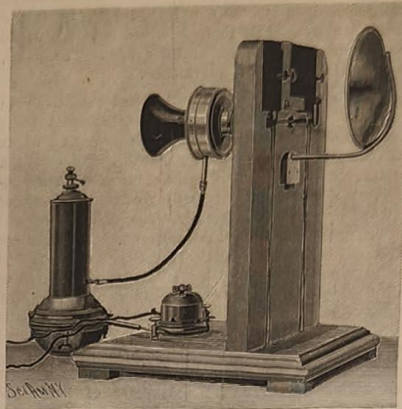
Fig. 1.—REFLECTOR TRANSMITTER OF RUHMER'S APPARATUS.
