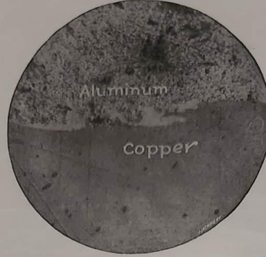
Fig. 6.—Microphotograph of a copper-aluminium weld. This shows a magnification of 850 times.
