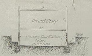
Fig. 2.—After alteration, with the cellar space made available for manufacturing operations.
