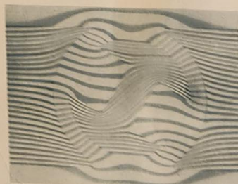
Fig. 6. Distortion of the "lines" just before maximum inductance.
