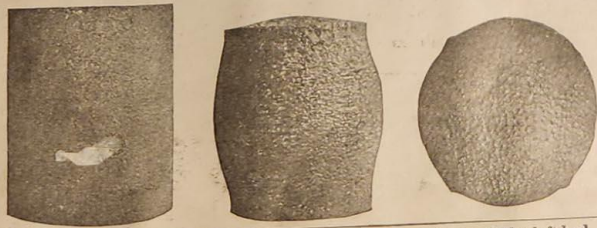
After 800 heatings and quenchings, the block of steel shown at the left had developed the shape at the right, passing through the central stage
