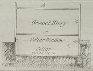
Fig. 1.—The original state of the building, with dark cellar space.
