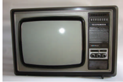
Color receiver, model TVC 364V, solid-state circuit topology, using "high-light" 14 inch series kinescope, made by Telefunken-Brazil in late Seventies.
