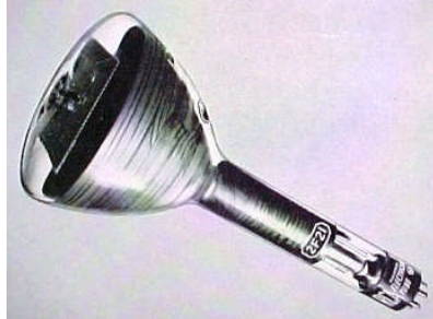
RCA 2F21 monoscope, part of TK-1A system.
