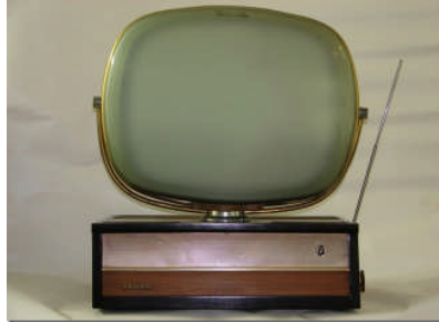
Black-and-white table TV set, "Predicta" model, made by Philco-Brazil based on the American counterpart, model UG-4242M. Tube circuitry using a 21-inch CRT, circa 1956.
