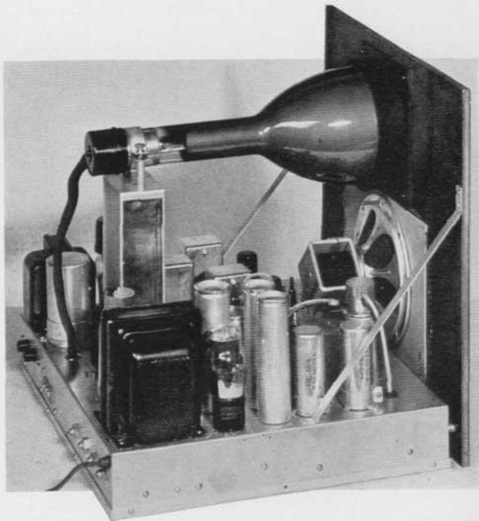
FIG. 46. SIDE VIEW OF THE ASSEMBLED SIGHT AND SOUND RECEIVER, WITH THE FIVE-INCH PICTURE TUBE MOUNTED AND READY TO OPERATE.
