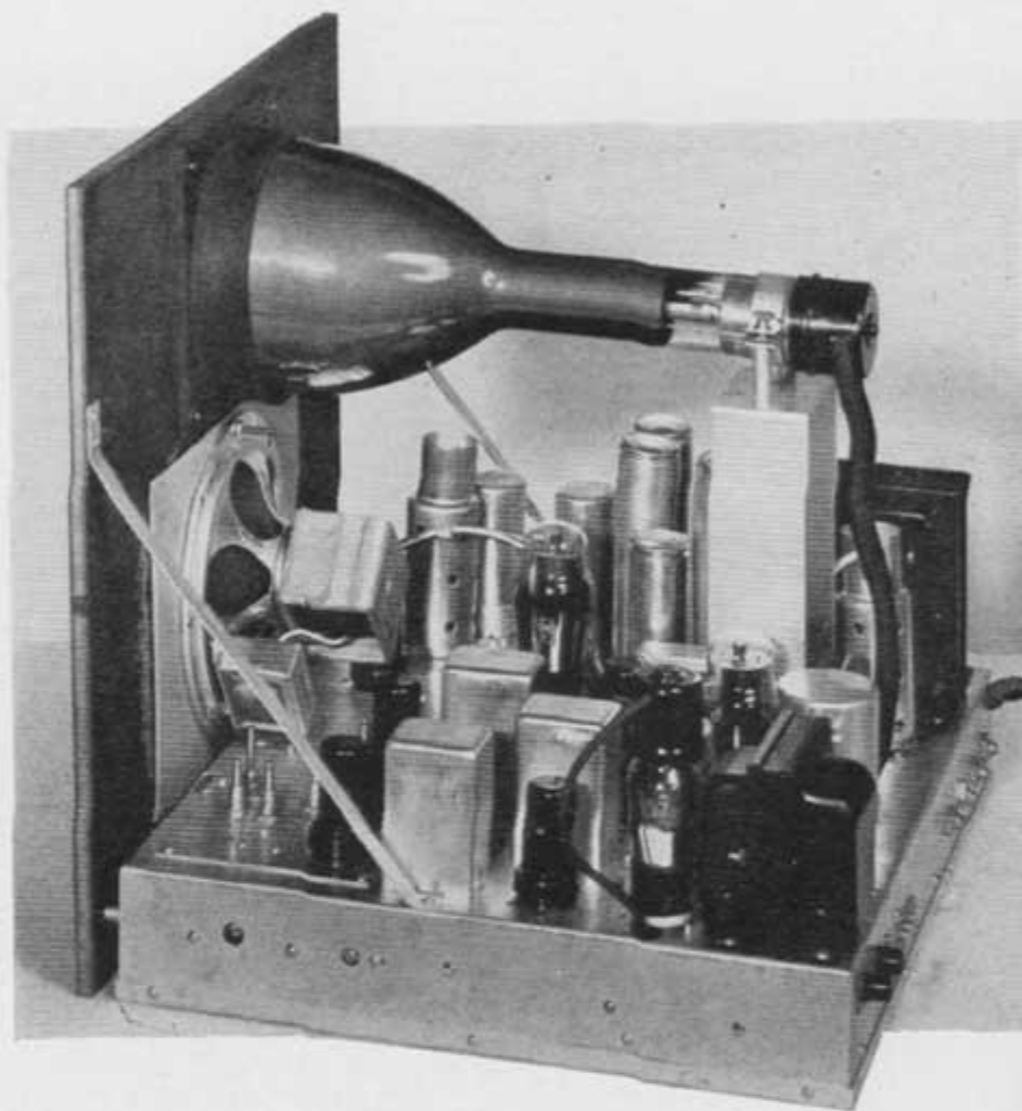
FIG. 57. COMPARING THE ASSEMBLY STAGE DRAWINGS WITH THE VIEWS OF THE ASSEMBLED CHASSIS WILL CLARIFY THE SUCCESSIVE CONSTRUCTION STEPS. NOTE THE HOLES IN THE SIDE OF THE CHASSIS, TOWARD THE FRONT, FOR ADJUSTING THE SOUND SENSITIVITY CONDENSER AND TRIMMER A.
