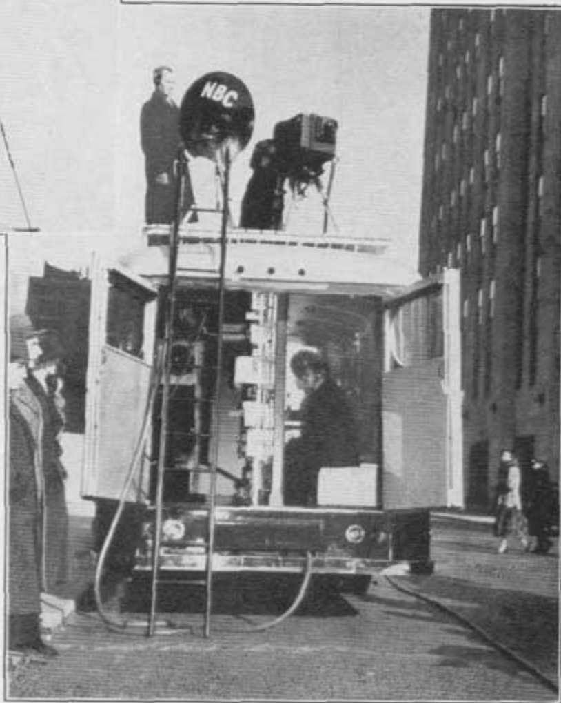
FIG. 40. A PLATFORM ON THE TOP OF THE PICK-UP UNIT OFFERS A POINT OF VANTAGE FOR THE CAMERA AND MICROPHONE. THE MONITORING OPERATOR CAN BE SEEN AT THE CONTROLS IN THE VAN. SPACE IS PROVIDED ON THE LEFT FOR THE CAMERA AND THE REELS OF COAXIAL CABLE REQUIRED FOR CONNECTIONS WHICH RUN OUT FROM THE TERMINALS BELOW THE DOORS.
