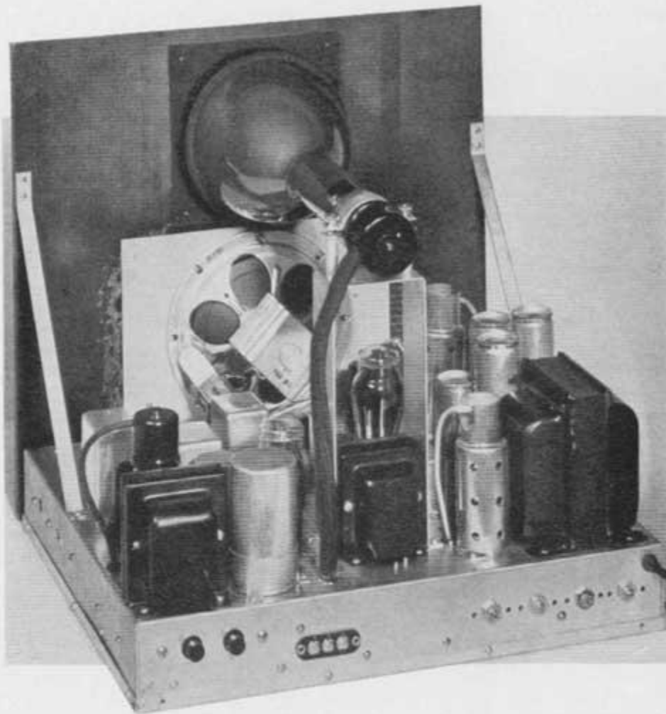
FIG. 47. REAR VIEW OF THE ANDREA RECEIVER. NOTE THE SURPRISING SIMPLICITY OF THE DESIGN. IT CAN BE ASSEMBLED IN LESS THAN TWELVE HOURS BY AN EXPERIENCED SET-BUILDER, BUT A BEGINNER MAY REQUIRE TWENTY-FOUR TO THIRTY HOURS.
