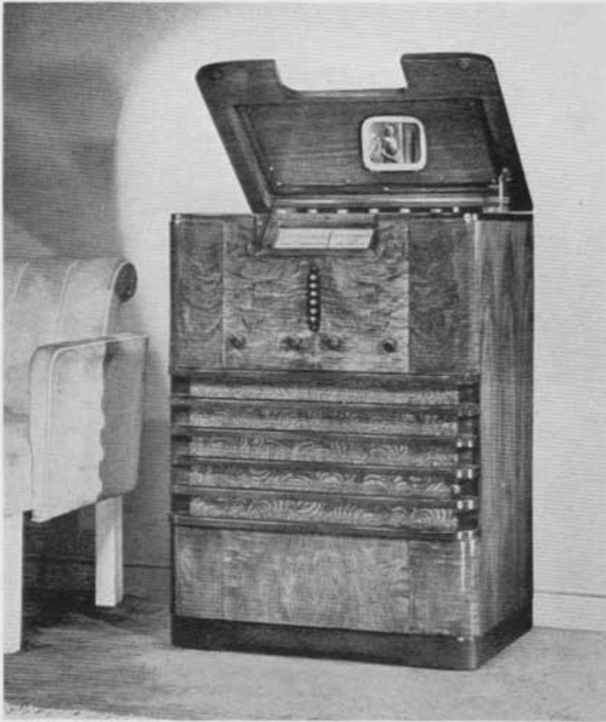
FIG. 24. THE ANDREA KT-E-5 CHASSIS CAN BE MOUNTED IN THIS MANNER FOR MIRROR VIEWING. CONTROLS AT THE TOP ARE FOR THE TELEVISION SET, AND AT THE FRONT, FOR AN ALL-WAVE SOUND RECEIVER. THIS MAKES A MOST ATTRACTIVE PIECE OF FURNITURE.
