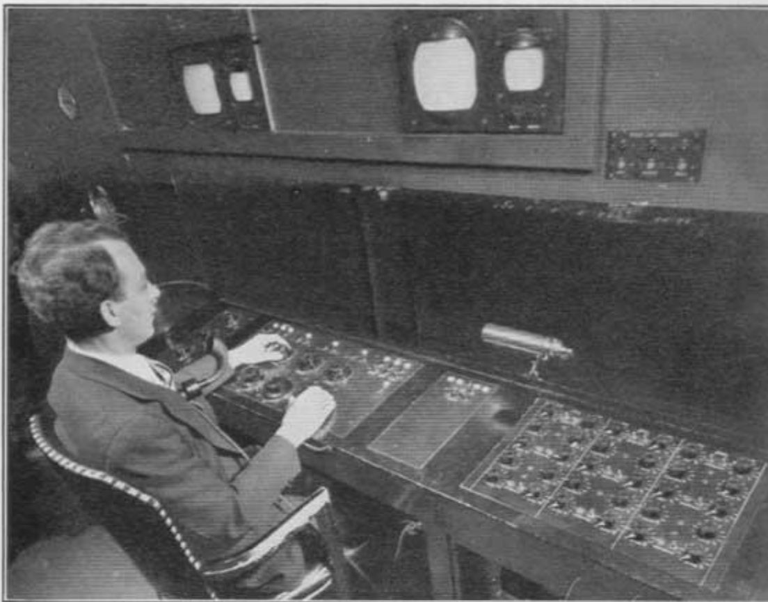
FIG. 32. MONITORING BOOTH, OVERLOOKING THE NBC TELEVISION STUDIO. THE OPERATOR, LOOKING THROUGH A GLASS PANEL, WATCHES THE ACTION, AND CHECKS THE PICK-UP IN THE PICTURE TUBE. DETAILS OF THE EQUIPMENT ARE GIVEN IN OTHER ILLUSTRATIONS.
