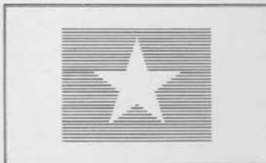
FIG. 16. FIRST RECEIVING INTERLACE, FORMED BY SCANNING EVERY OTHER LINE. INTERLACED SCANNING ELIMINATES FLICKER.
