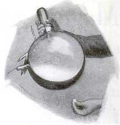
Two extremes in photo-electric cells—the eleven-inch bulb made by L. T. Garner, University of Illinois, is said to be the world's largest. The other cell is an ordinary-sized one.
