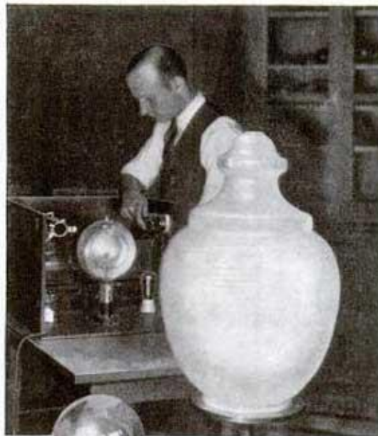
A photo-electric cell apparatus for measuring the light-transmitting properties of ornamental glass globes for street lamps—in use by General Electric Company.
