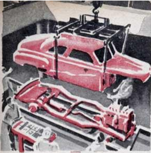
Remote control matches the pace of merging assembly lines, as where body of a car meets chassis.
