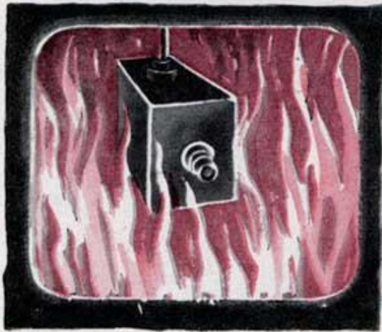
Television cameras with cooling jackets can disclose what happens in smelters, glass furnaces and other places where terrific heat precludes a direct view.
