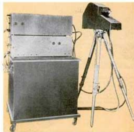
Here is the portable television camera and the amplifier used with it.
