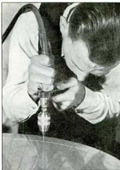
In drilling the scanning disk, hairlike No. 76 drills were used. Care was taken to keep the drill vertical.
