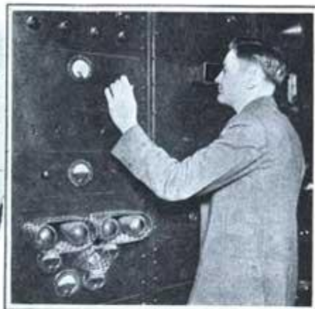
Television's control board. Here the operator is looking into the monitor which reproduces image.
