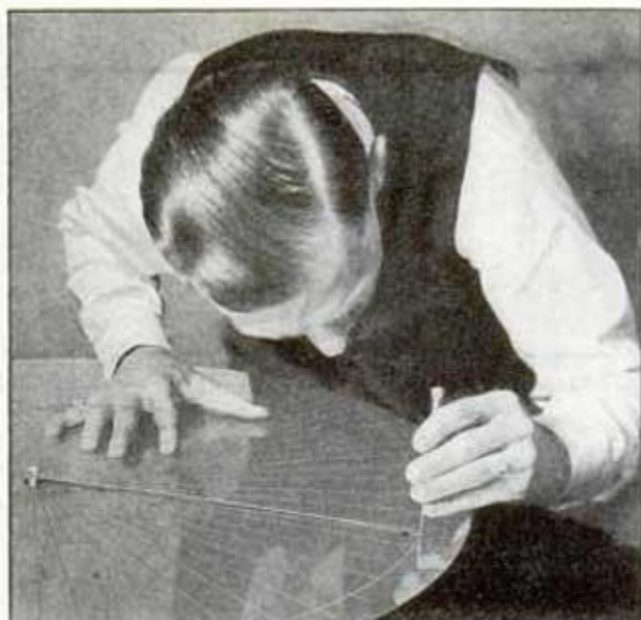
Above: Scribing the spiral by wrapping the wire around a \frac{3}{4} -in. stud. At right: A \frac{1}{2} -in. lathe faceplate, drilled through, is used as a hub for the disk. Below: A \frac{3}{8} to \frac{1}{2} in. bushing is inserted in the faceplate to take the \frac{3}{4} -in. stud.
