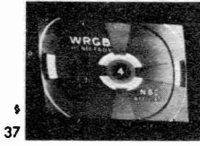
37 FAULT —Rhombus picture reduction in Height and Width. CAUSE —Yoke does not contain three (of four) ferrite Yoke segments.
