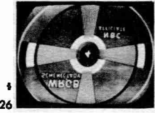
26 FAULT —Reverse and Upside Down Picture. CAUSE —Wires going to vertical section of Yoke are reversed.
