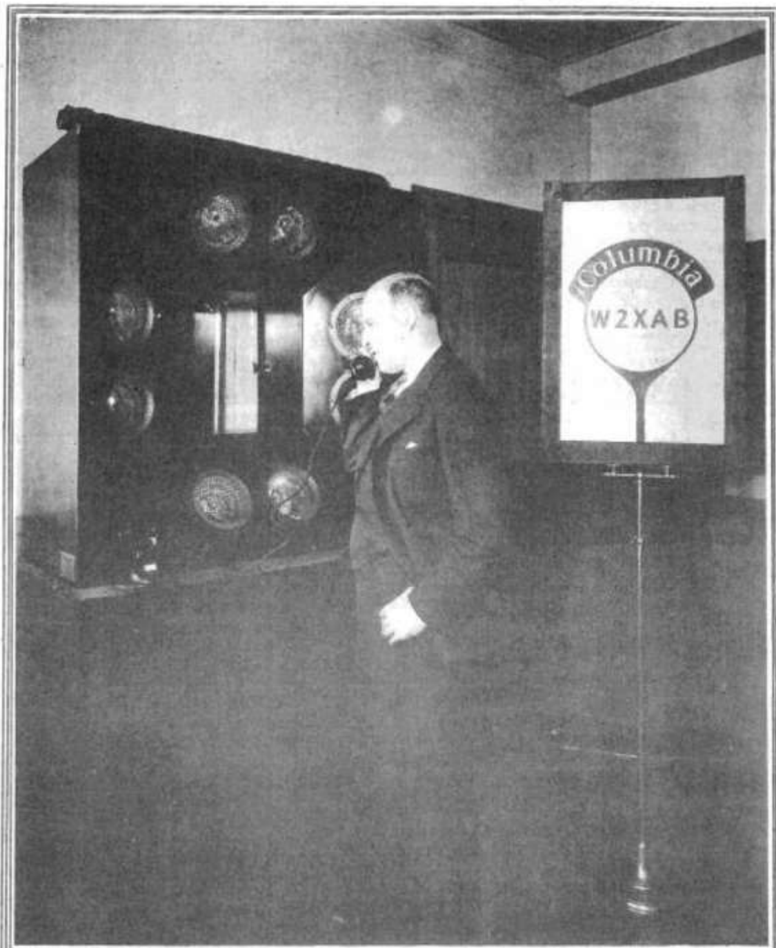
THE PHOTOELECTRIC CELLS ARE SPREAD IN A WIDE BANK WHEN THE FLYING-SPOT IS USED FOR SCANNING.
