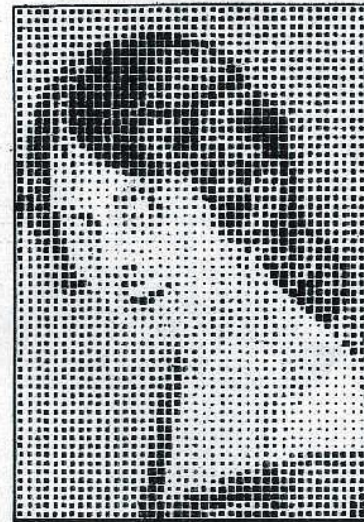
Fig. 16. Example of code transmission varying the size of the dark areas of the square, the total number of squares remaining exactly as before.
