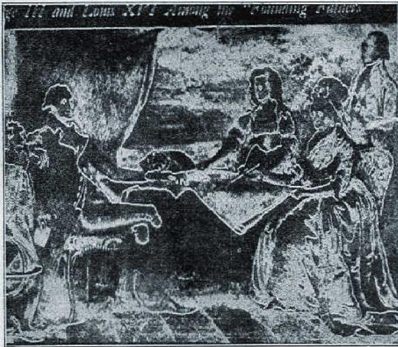
Fig. 77. This distorted picture was made from a newspaper reproduction of a steel engraving of "Washington's Family" by E. Savage. The distortion is due to the improper adjustment of the receiver apparatus. This picture may serve to give a visual idea of the audible distortion sometimes experienced by broadcast listeners.
